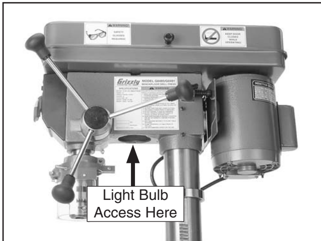
Figure 20. Light bulb access location.
